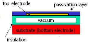
**FIGURE 1.** A simplified cross-section of a CMUT.
